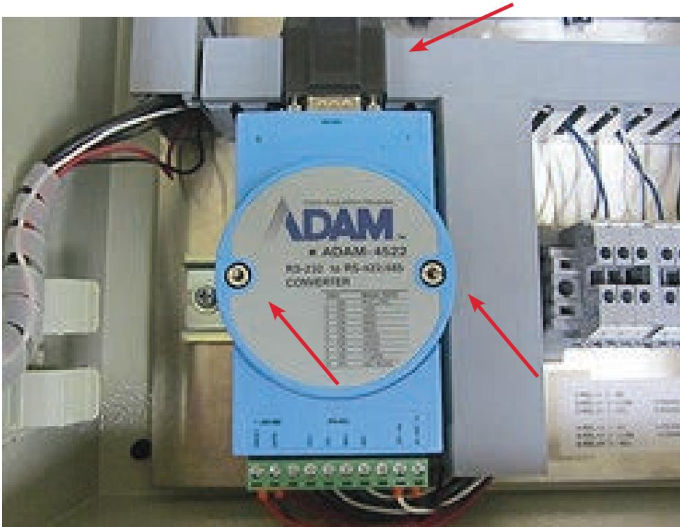
ii. Lift the ADAM-4522 module out of the way to expose the ADAM 4069 module beneath.
