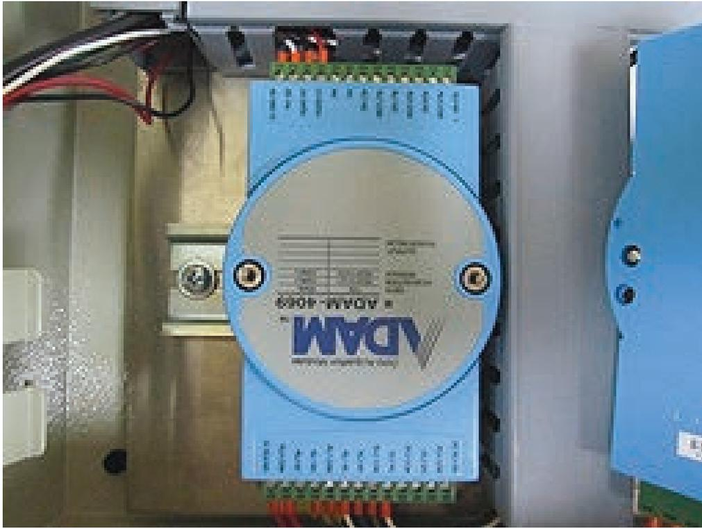
iii. The ADAM-4069 module has 4 available Form-A (SPST) Normally Open relays available and 1 Form-C (SPDT) terminal strips on the top and bottom connector. Relays 4, 5 and 6 are Form-A; relay 7 is Form-C.
