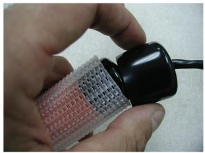
**Note:** The EEC should be inspected monthly for blockage. If the mesh tube becomes contaminated with dirt or debris, it could prevent a leak from being detected rapidly. To clean the EEC, remove the cap, carefully remove the FFS, and wash the EEC in water or IPA (do not remove screen!). FFS cleaning (if necessary) is a separate operation, please refer to TT-FFS Fast Fuel Detection Probe Care and Cleaning Instructions (H58307).
